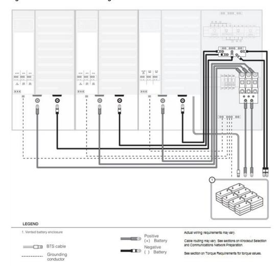
Figure 48 Three-Phase DC Wiring
