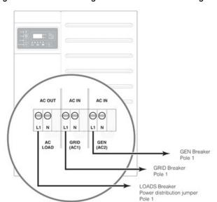
Figure 49 Inverter/Charger Three-Phase AC Wiring
