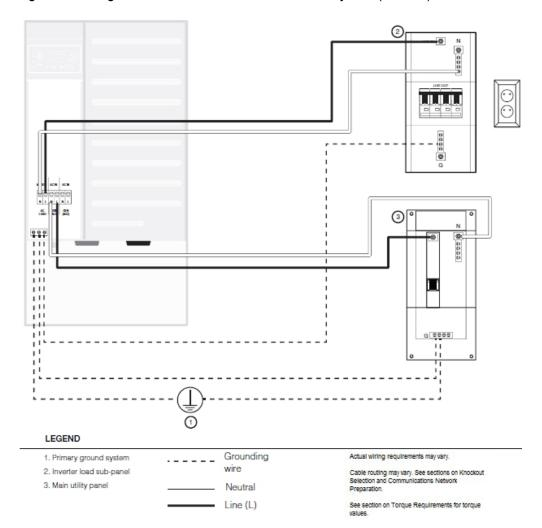
Figure 37 Wiring to the Inverter Load Sub-Panel or Utility Grid (no PDP)
