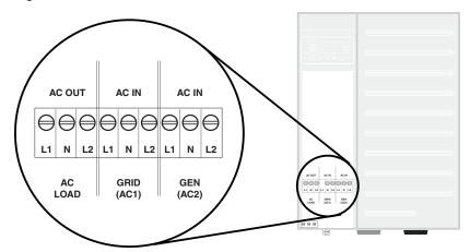
The neutral inputs are connected to each other, requiring only one neutral connection when installed with a Power Distribution Panel (PDP). Without the PDP, additional neutral connections may be required at the input sources.
