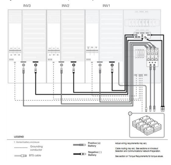
Figure 47 DC Connections for a Triple-Inverter System
