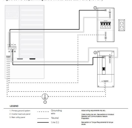
Figure 53 AC Output Wiring to the Inverter Load Sub-Panel (No PDP)
