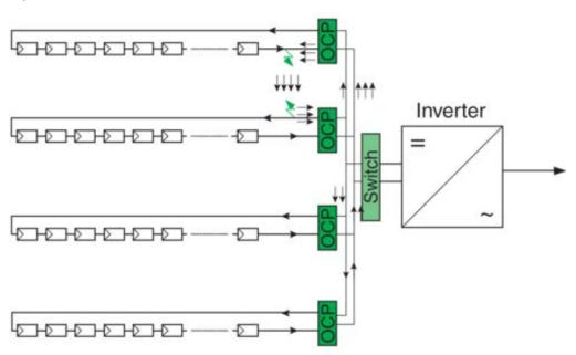
Selected insulation monitoring devices or overcurrent protection in earthed systems must detect the first fault and staff must address the first fault and clear it without delay.
