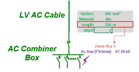
The example above results in around 7.20 kA. Generally, we see the fault level on AC Combiner buses within the range of 10 to 20 kA. For this application, we recommend using breakers in the NG125N category or higher to help ensure a minimum of 25 kA fault current rating at the AC combiner level.
