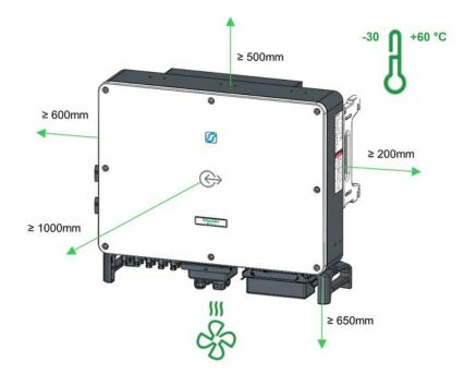
Figure 24 Installation space between inverters
