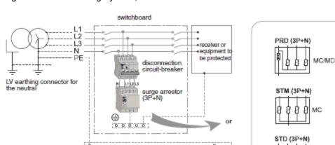
Figure 17 TN-S Earthing System, 3-Phase + Neutral
