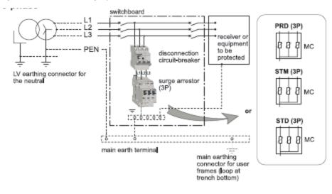
Figure 18 TN-C Earthing System, 3-Phase
