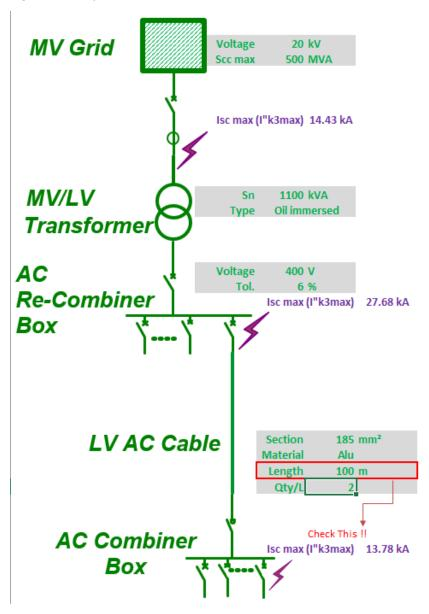
The example circuit in *Figure 9* has 100 m length from the AC combiner to the AC recombiner. The resulting fault level at the AC combiner bus bar is 13.78 kA and the choice of breaker is NG125N MCCB (25 kA). Figure 10 Example circuit with 250 m cable
