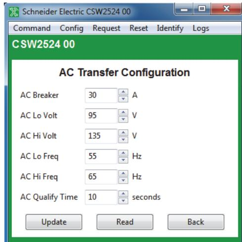
**Figure 3-24** Inverter/Charger AC Transfer Configuration
