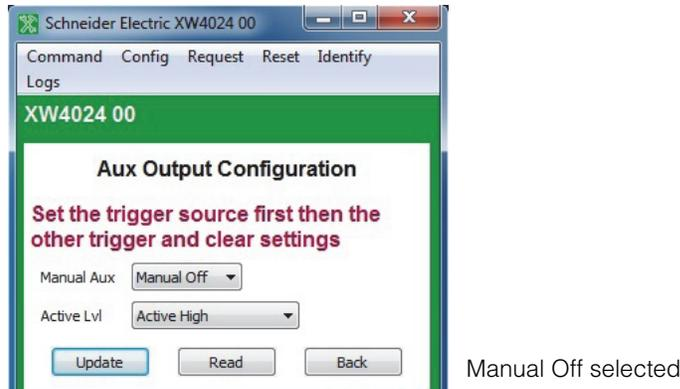
**Figure 3-14** Inverter/Charger Aux Output Configuration
