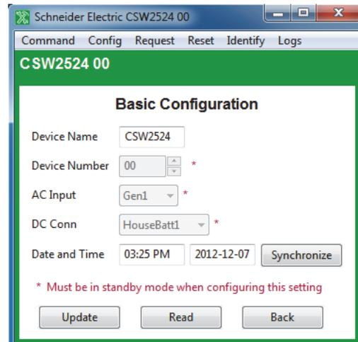
**Figure 3-21** Inverter/Charger Basic Configuration
