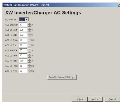
**Figure 2-37** Xantrex XW Inverter/Charger AC Settings
