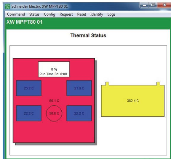
Figure 3-29 Viewing Thermal Status (MPPT 80 Only)
