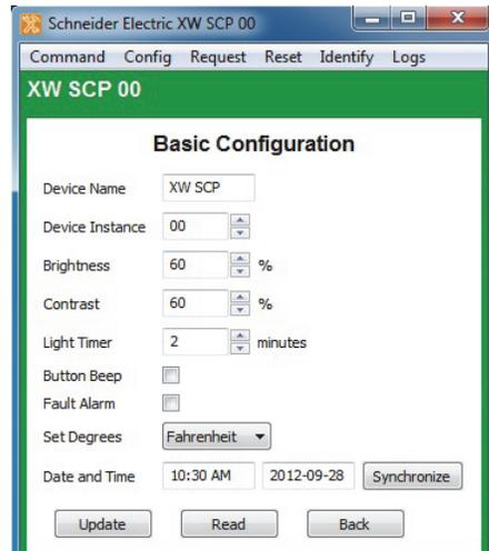
**Figure 3-49** SCP Basic Configuration
