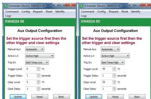
Figure 3-15 Inverter/Charger Aux Output Configuration (Batt Temp Triggers)
