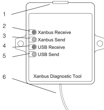
**Figure 1-4** USB-to-Xantrex Xanbus adapter
