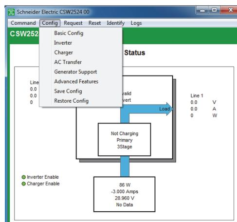
**Figure 3-19** Conext SW Inverter/Charger Config Menu
