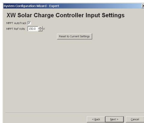
**Figure 2-43** Xantrex XW Solar Charge Controller Input Settings**Table 2-12** Xantrex XW Solar Charge Controller Input Settings
