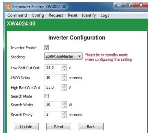
**Figure 3-9** Inverter/Charger Inverter Configuration
