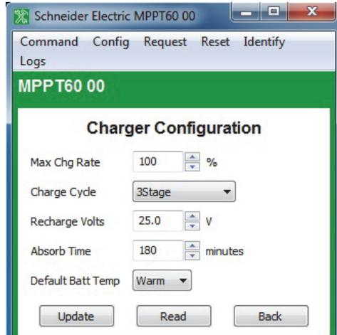
**Figure 3-31** Charge Controller Charger Configuration
