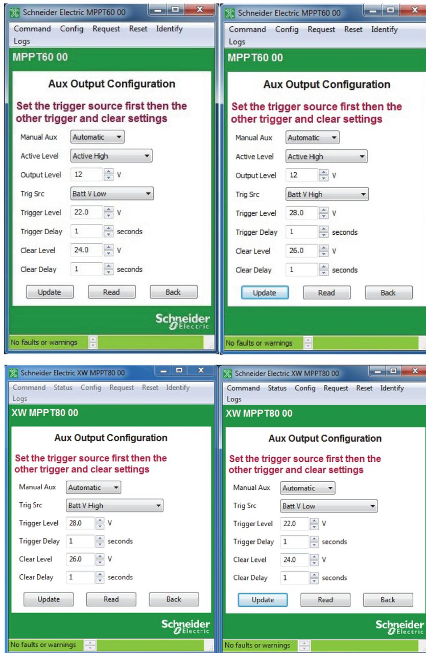
Figure 3-36 Charge Controller Aux Output Configuration (Batt Voltage Triggers)
