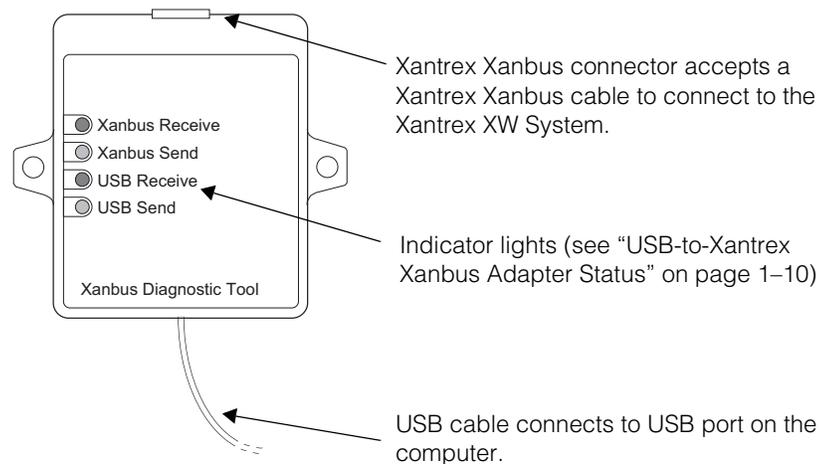
**Figure 1-1** USB-to-Xantrex Xanbus adapter
