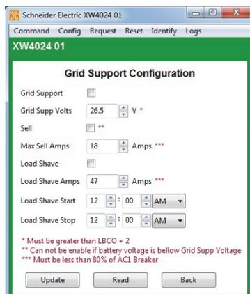
**Figure 3-12** Inverter/Charger Grid Support Configuration
