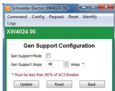
**Figure 3-13** Inverter/Charger Gen Support Configuration
