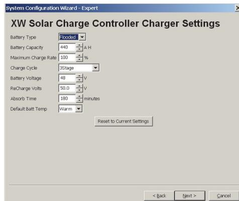
**Figure 2-41** Xantrex XW Solar Charge Controller Charger Settings
