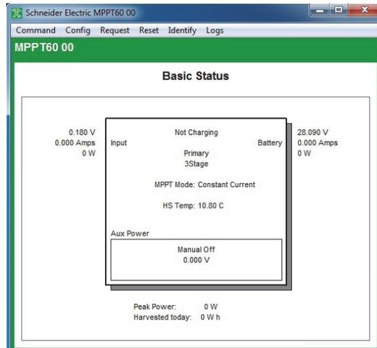
Figure 3-28 Charge Controller Basic Status
