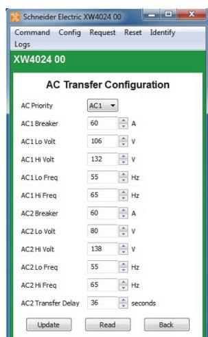
**Figure 3-11** Inverter/Charger AC Transfer Configuration
