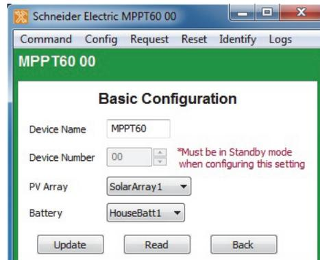
**Figure 3-30** Charge Controller Basic Configuration
