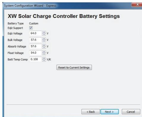
**Figure 2-42** Xantrex XW Solar Charge Controller Custom Battery Settings
