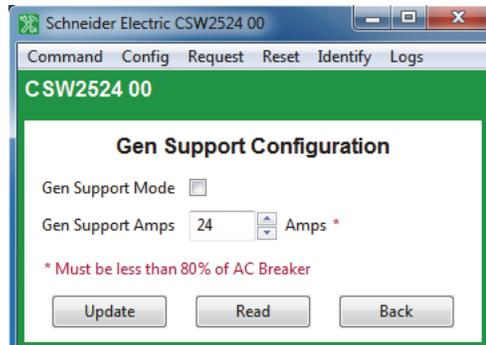
**Figure 3-25** Inverter/Charger Gen Support Configuration
