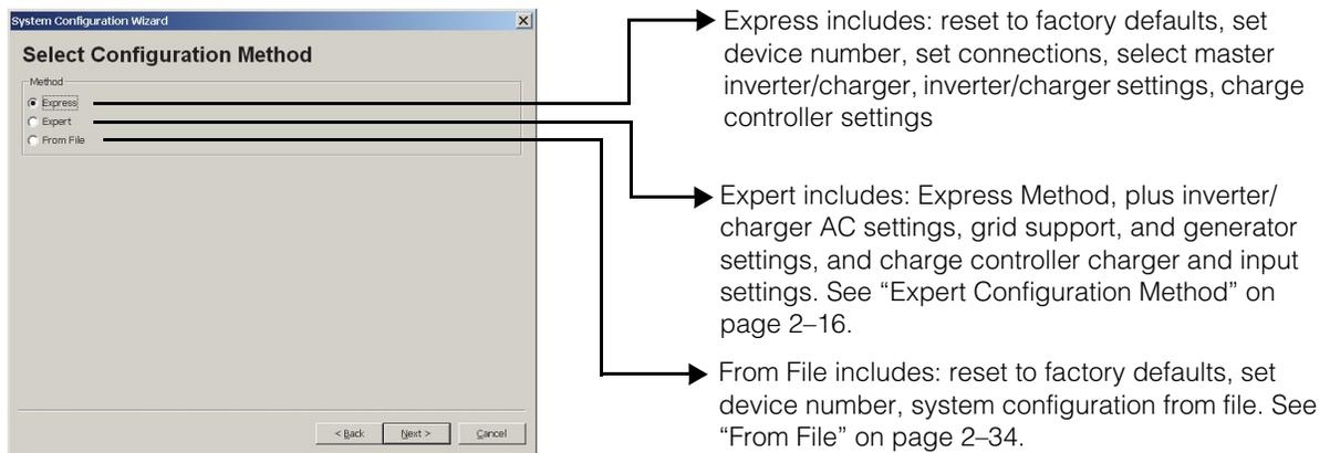
**Figure 2-3** Select Configuration Method
