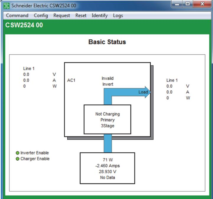
Figure 3-20 Conext SW Basic Status Window
