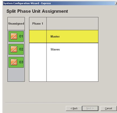
**Figure 2-8** Split-Phase Unit Assignment
