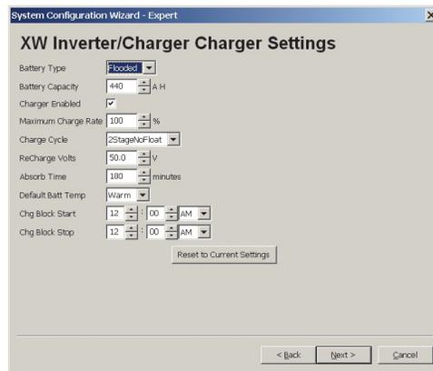
**Figure 2-35** Xantrex XW Inverter/Charger Charger Settings
