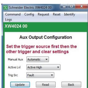
Figure 3-17 Inverter/Charger Aux Output Configuration (Fault Trigger)
