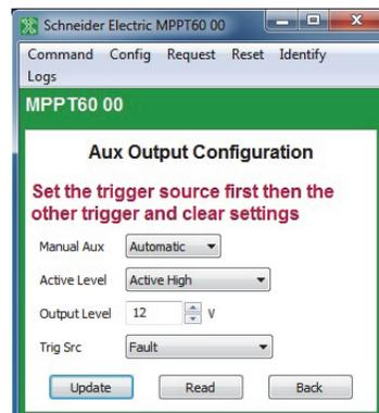
Figure 3-39 Charge Controller Aux Output Configuration (Fault Trigger)
