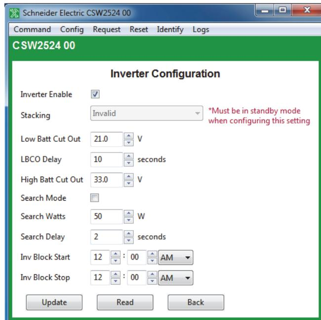
Figure 3-22 Inverter/Charger Inverter Configuration
