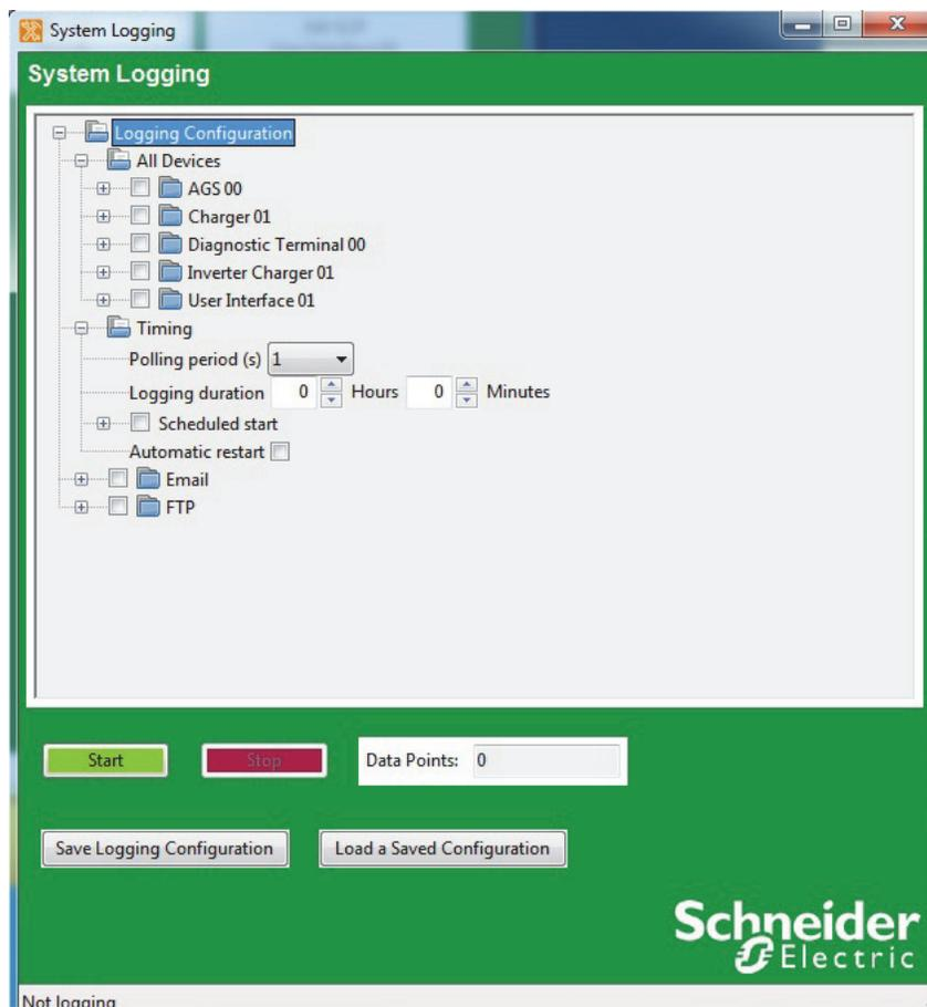
Figure 4-1 System Logging Window
