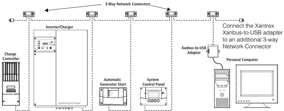
Figure 1-3 Multi-drop Backbone Layout
