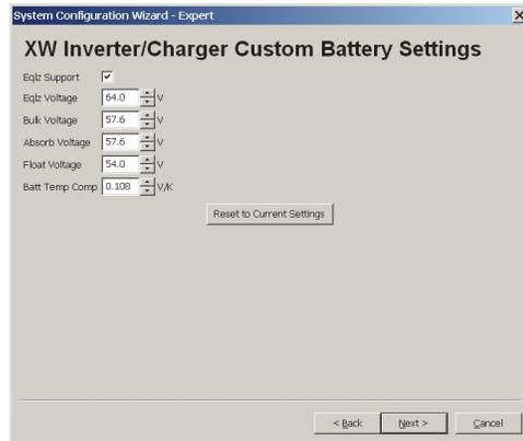
**Figure 2-36** Xantrex XW Inverter/Charger Custom Battery Settings
