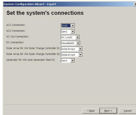
**Figure 2-26** System Connections
