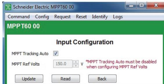
**Figure 3-33** Charge Controller Input Configuration
