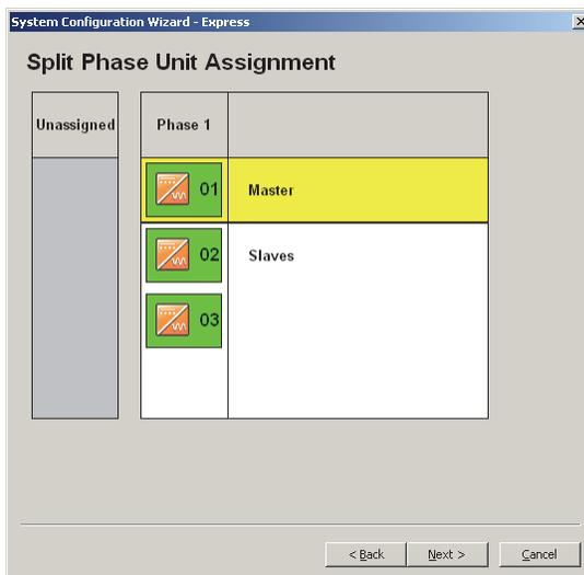
**Figure 2-9** Assigning Split-Phase Units
