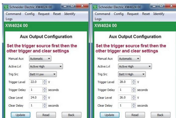
Figure 3-16 Inverter/Charger Aux Output Configuration (Batt Voltage Triggers)
