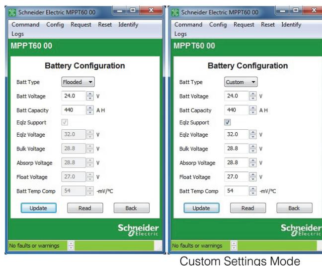
Figure 3-32 Charge Controller Battery Configuration
