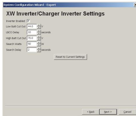
**Figure 2-34** Xantrex XW Inverter/Charger Inverter Settings
