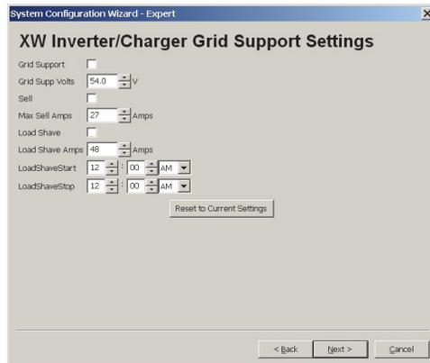
Figure 2-39 Xantrex XW Inverter/Charger Grid Support Settings
