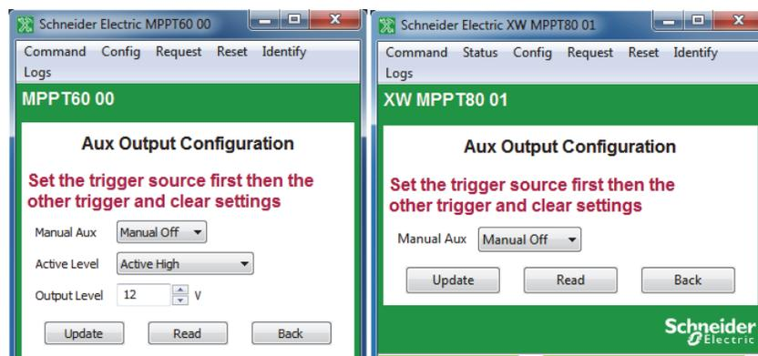
**Figure 3-35** Charge Controller Aux Output Configuration (ManualOff)
