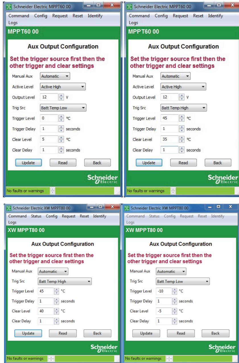
Figure 3-37 Charge Controller Aux Output Configuration (Batt Temp Triggers)
