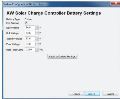
**Figure 2-18** Charge Controller Custom Battery Settings
