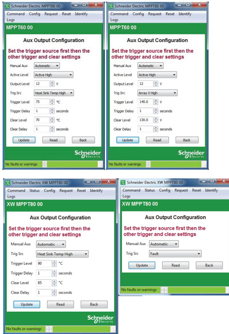
**Figure 3-38** Charge Controller Aux Output Configuration (Heat Sink and Array Voltage Triggers)
