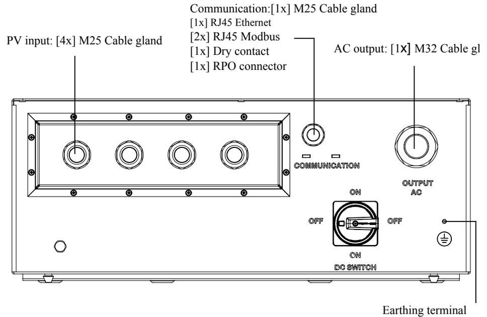
Figure 1-6 Bottom view of the wiring box
