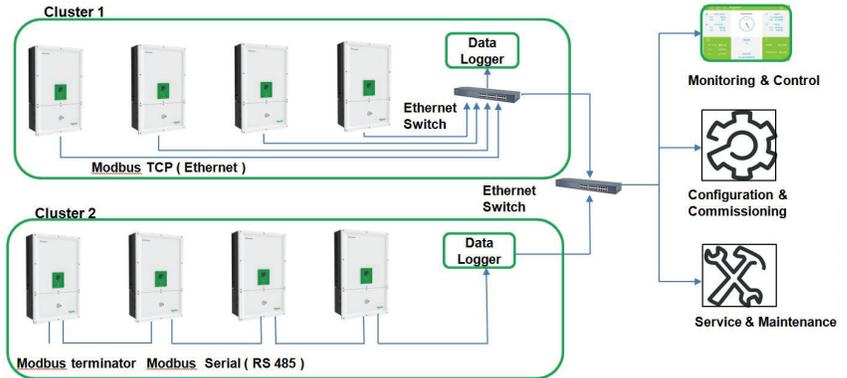
Figure 2-49 Cluster 1: Modbus TCP and Cluster 2: Modbus RS485 connections
