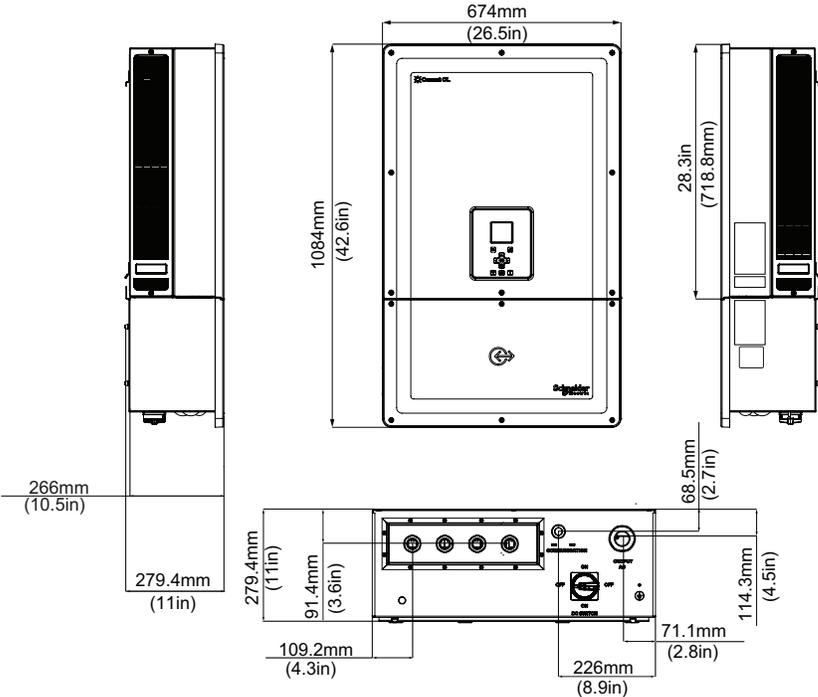
Figure 2-9 Views and dimensions of the inverter and the wiring box (Essential/Optimum)
