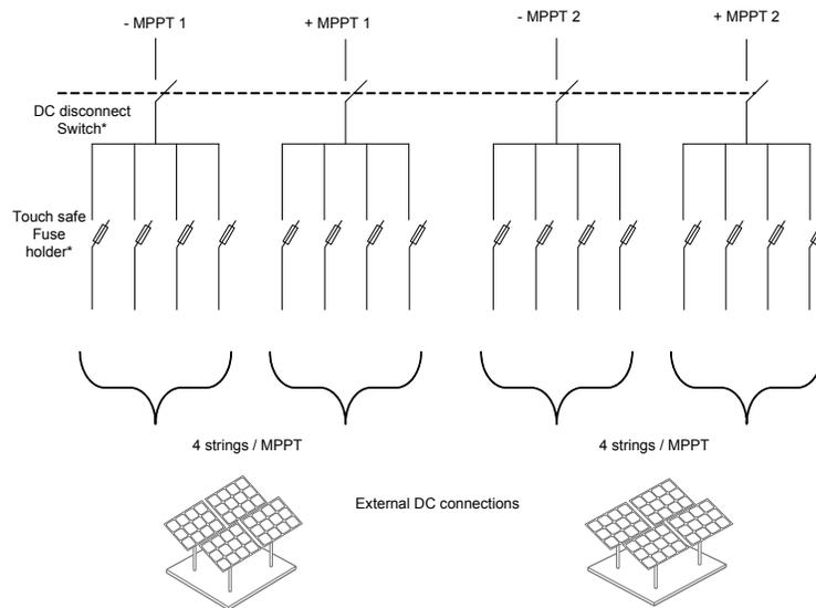
Figure 2-33 PV Wiring diagram of Conext™ CL 20000E and 25000E models
