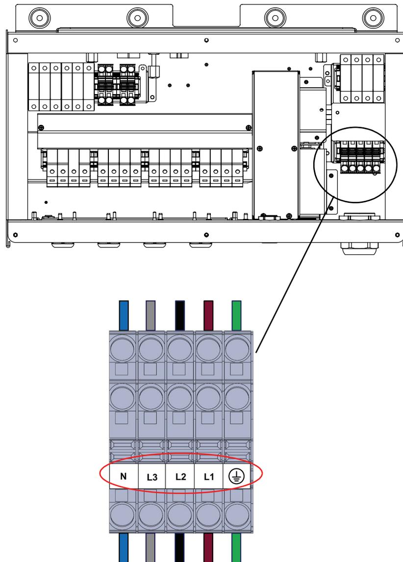
Figure 2-36 **Wire installation**
