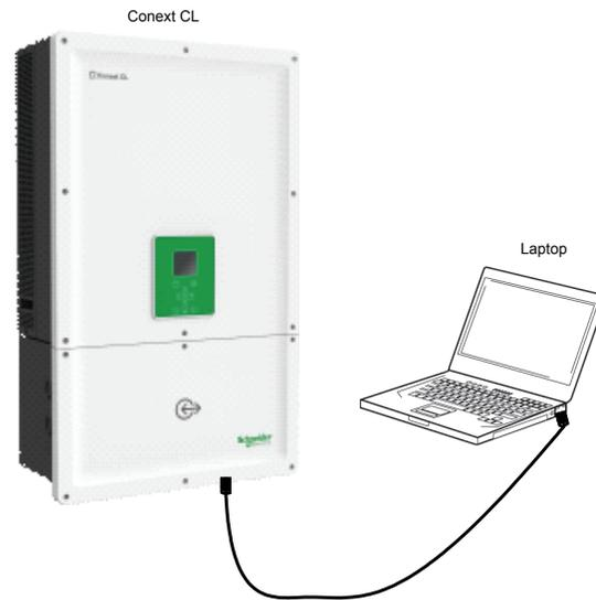
Figure 2-57 **Web Interface connection** diagram
