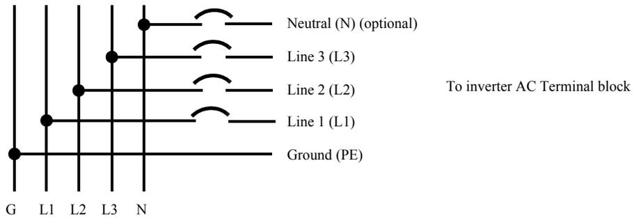
Figure 2-38 AC connection details
