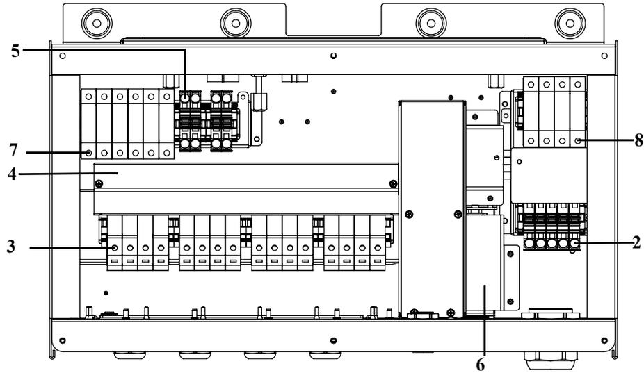
Figure 2-13 **Wiring box- Optimum (PVSC2025E300)**
