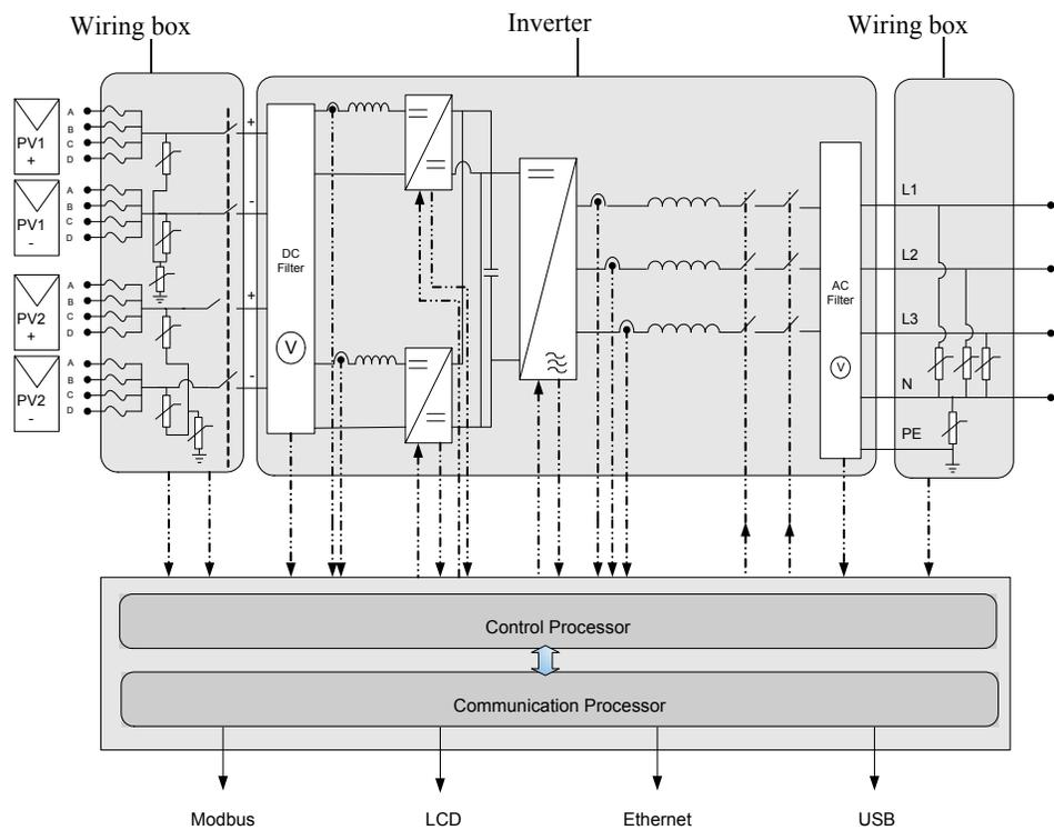
Figure 1-2 Block diagram of Conext™ CL 20000E and 25000E models
