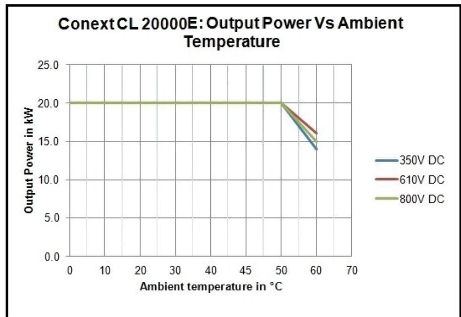
Figure A-3 Derating curve- 20kW
