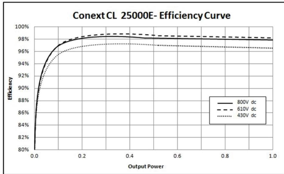
Figure A-2 Efficiency curve- 25kW
