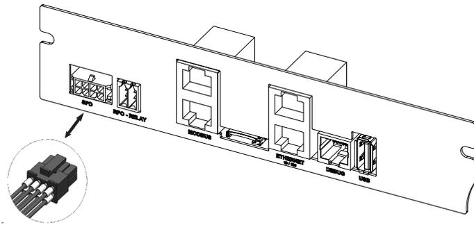
Figure 2-43 SPD monitoring cable connection
