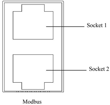
Figure 2-44 Modbus (RS485) connectors
