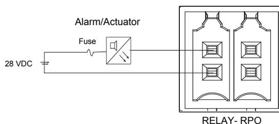
Figure 2-51 **Dry Contact Relay connection**
