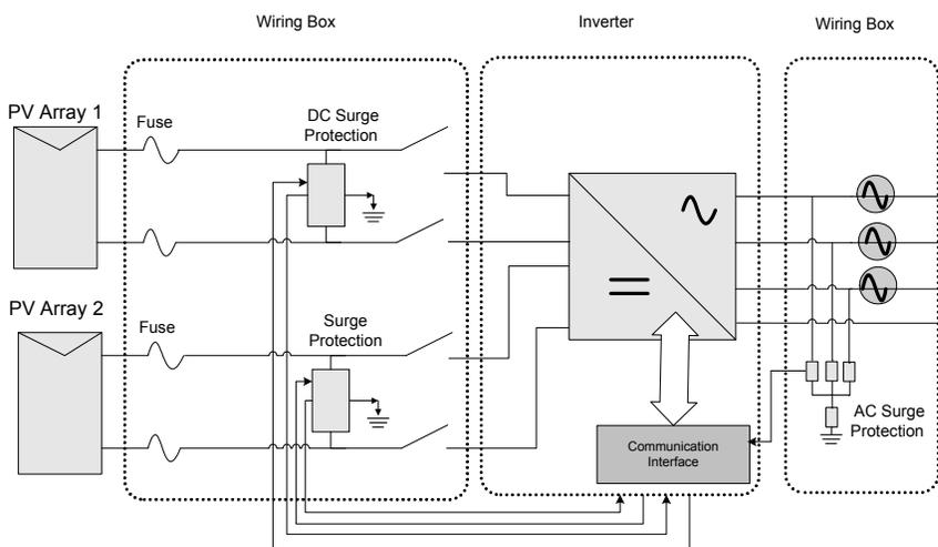
Figure 2-55 Surge Protection device wiring
