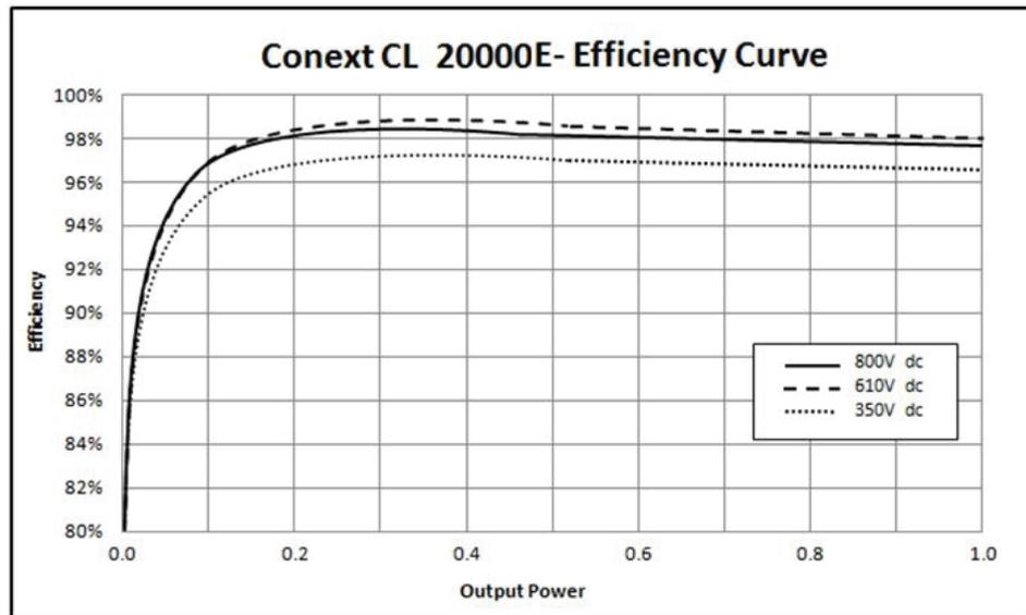
Figure A-1 Efficiency curve - 20kW
