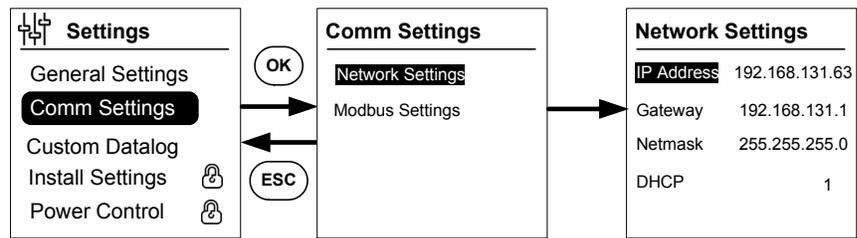
Figure 2-45 Checking the IP address
