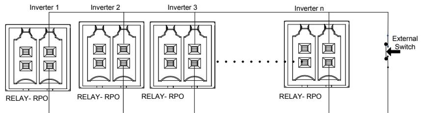
Figure 2-54 RPO connection with multiple inverters
