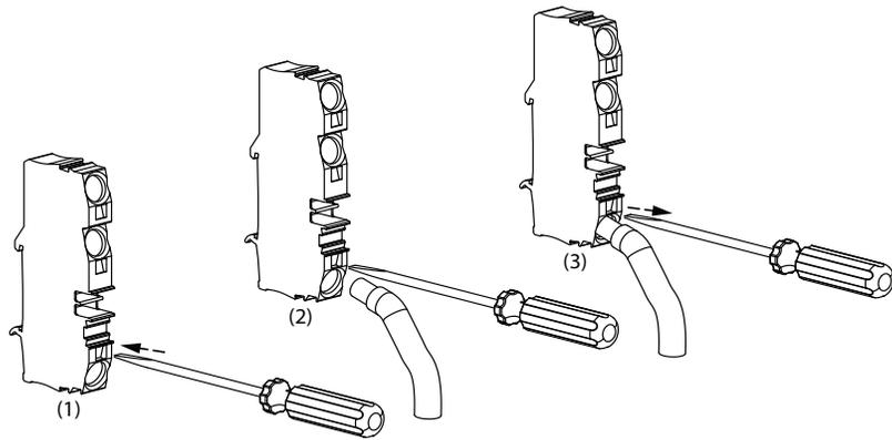
Figure 2-37 Wire installation
