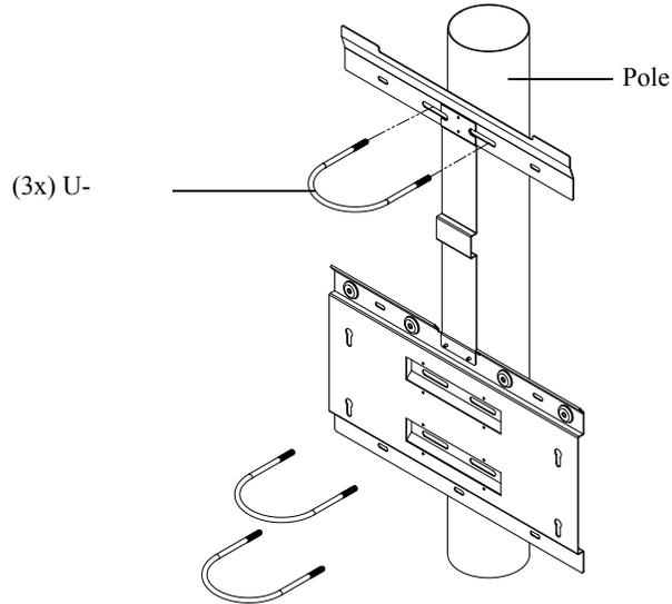
Figure 2-19 Front view of the pole mounting installation
