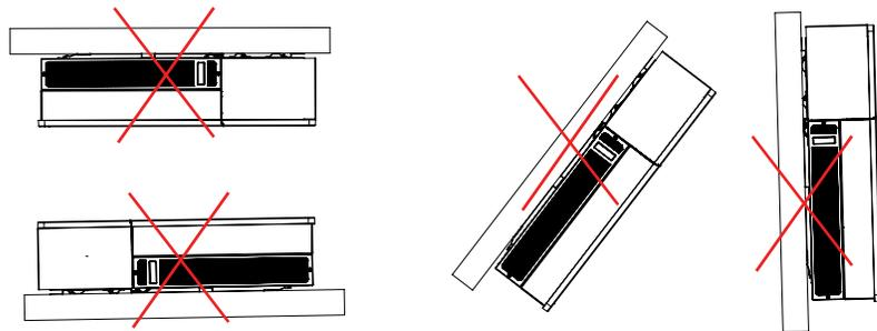
Figure 2-7 Incorrect mounting positions
