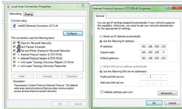
Figure 2-47 Ethernet Connection
