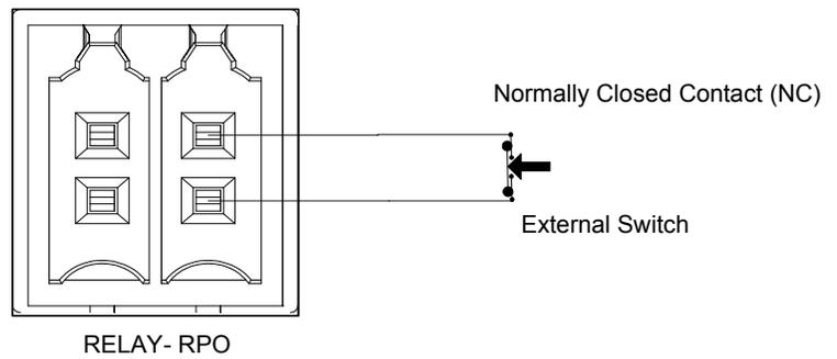
Figure 2-53 RPO connection for single inverter
