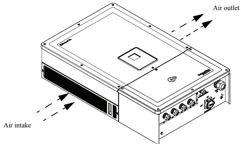
Figure 1-5 Cooling arrangement of the inverter
