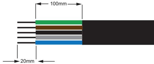
Figure 2-39 AC wiring
