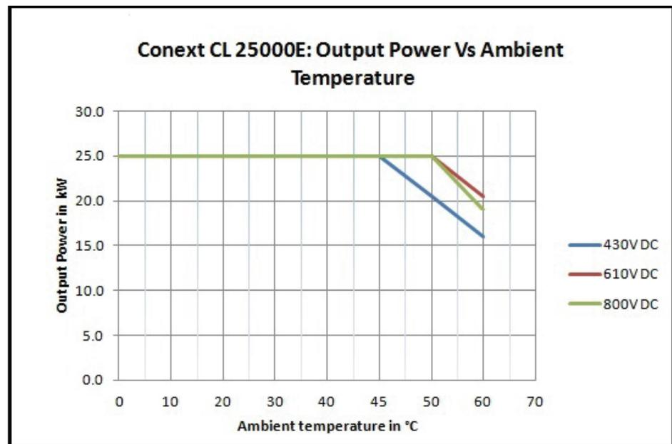
Figure A-4 Derating curve- 25kW
