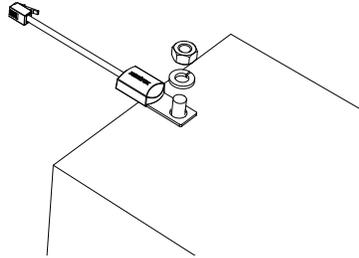
4. If connecting to the battery terminal, make sure the BTS does not prevent the power wiring from making the best possible contact with the battery terminal. If using the adhesive backing, install the BTS on the side of the battery below the electrolyte level. It is best to place the sensor between batteries and place the batteries in an insulated box to reduce the influence of the ambient temperature outside the battery enclosure.
