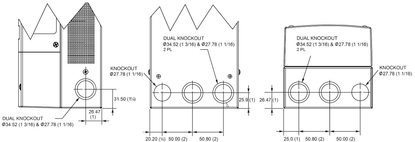
Figure 4 Dimensions and knockout locations
