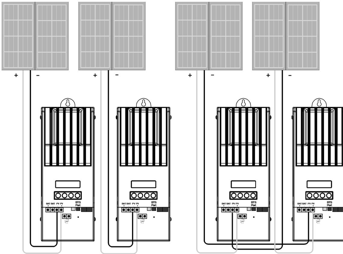
**Left:** Correct wiring —no interconnection between systems
