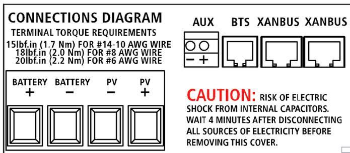
A label providing details on each connector and torque requirements for each terminal is affixed to the inside of the wiring compartment cover plate.
