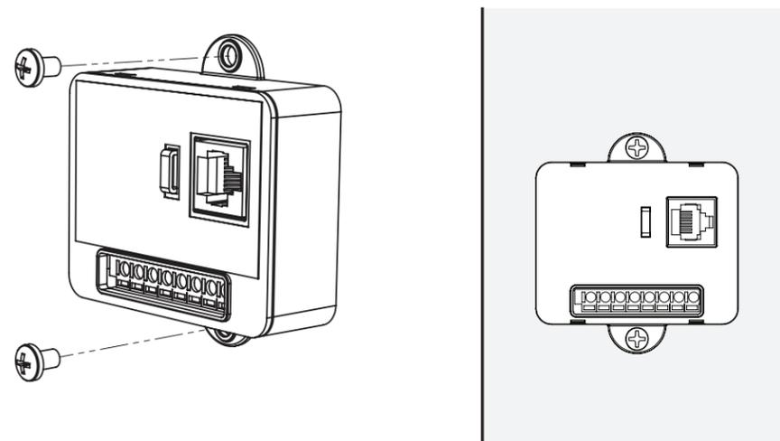
**E2 Battery Shunt Mounting**
