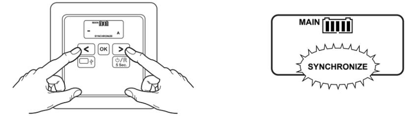
**NOTE:** Before synchronizing the Battery Monitor to a state of charge of 100%, charge the batteries completely and allow the batteries to remain in float state for two hours or longer after first installation.
