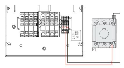
b. Connect a wire from the RS terminal #4 to the RS Initiator switch's top right terminal.
