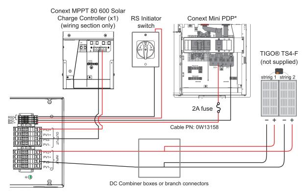
\*Connect the Bat+ and Bat- cables to the DC terminals in the Conext Power Distribution Panel (PDP), or the Conext Mini PDP. For details, see the Conext Power Distribution Panel Installation Guide (document number 975-0709-01-01) or the Conext Mini Power Distribution Panel Installation Guide (document number 975-0735-01-01).
