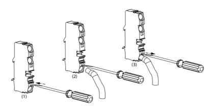
Figure 14 MPPT Disconnect RS connections
