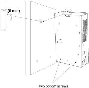
**Note:** If not attached to studs, you will need to provide adequate support for the MPPT Disconnect RS. For example, a sheet of plywood can be attached to the wall, and the MPPT Disconnect RS can then be attached to the plywood.
