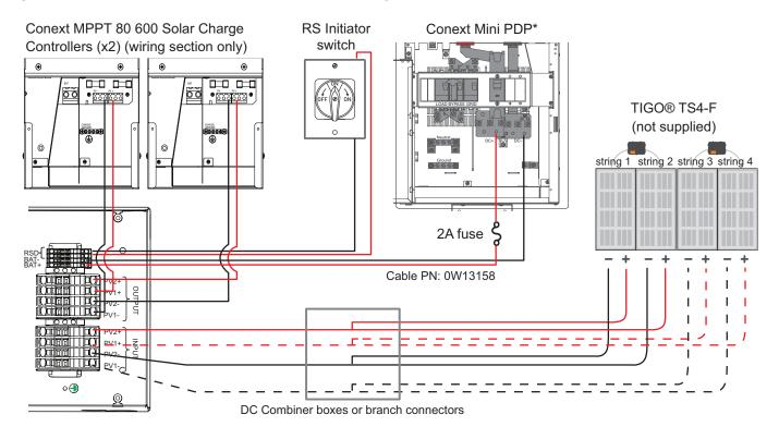
Figure 9 Connection to a single Conext MPPT 80 600 Solar Charge Controller
