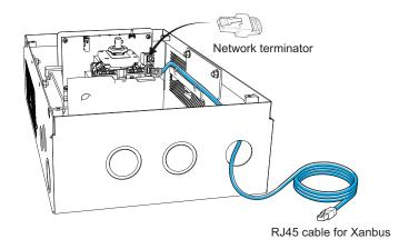
In a daisy chain layout, each device on the network is linked with separate lengths of cable, as shown in the figure below. The maximum number of Xanbus devices that can be connected is 15, with a baud rate of 256 kbps, and the maximum length is approximately 1000 m.
