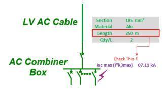
The example above results in around 7.11 kA. Generally, we see the fault level on AC Combiner buses within the range of 10 to 20 kA. For this application, we recommend using breakers in the NG125N category or higher to help ensure a minimum of 25 kA fault current rating at the AC combiner level.
