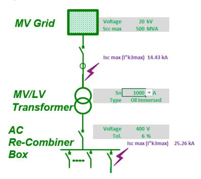
When we replace the 1000 kVA transformer with a 800 KVA transformer, the fault level decreases significantly on the AC re-combiner's bus bar and NSX400N type breakers become eligible to be used for inputs.
