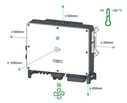
Figure 24 Installation space between inverters
