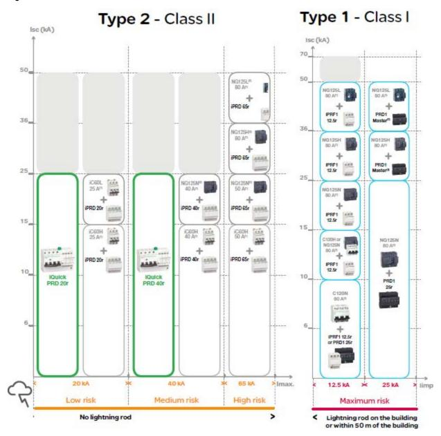
Figure 16 Coordination of SPDs with disconnection devices
