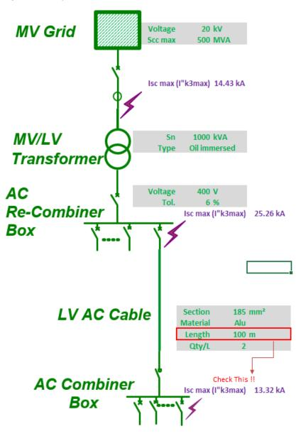
The example circuit in *Figure* 9 has 100 m length from the AC combiner to the AC recombiner. The resulting fault level at the AC combiner bus bar is 13.32 kA and the choice of breaker is NG125N MCCB (25 kA).
