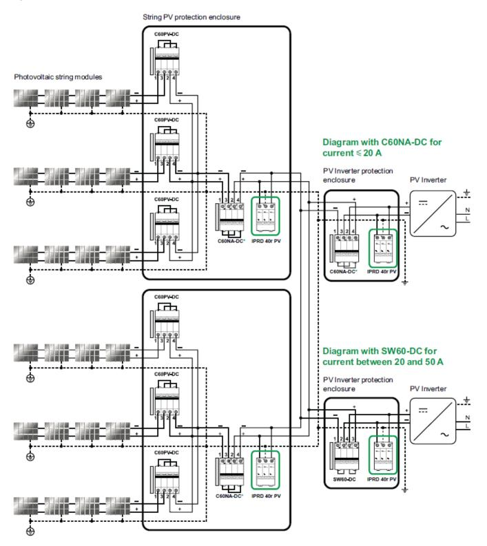
If there is a scenario where the PV architecture is without an earthed polarity on the DC side and with either a PV inverter or galvanic isolation, the following things are required:
