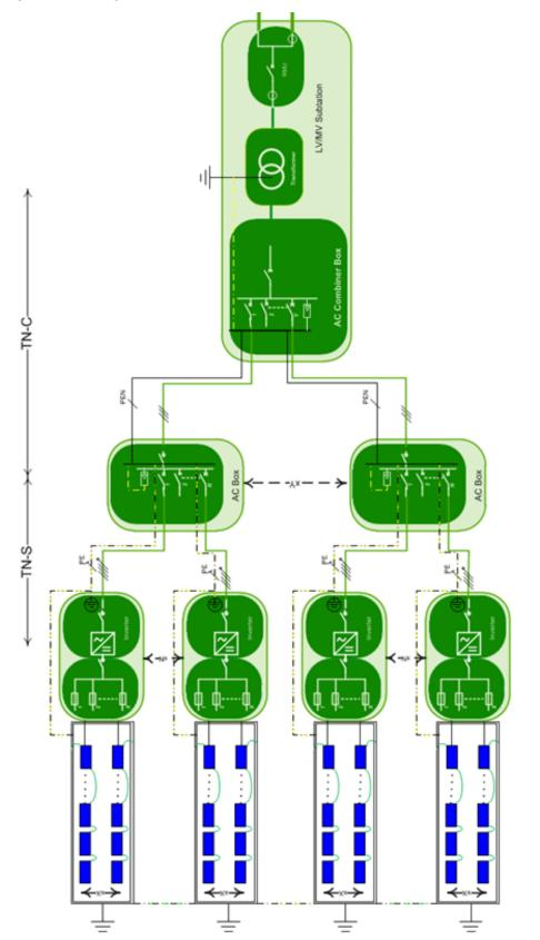
Country and area installation codes for earthing PV systems must be followed when sizing the earthing conductor. Selection of system components like SPDs, MCCB and MCB, disconnect switches, panel enclosures, and cables should be in accordance with the type of
