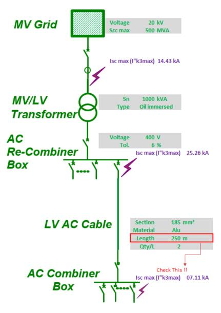
The example circuit in *Figure 10* has a 250 m length from the AC combiner to the AC recombiner, and the fault current is reduced to 7.11 kA, allowing the selection of C120H MCB with 15 kA fault level.
