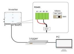
For designing the communication architecture, we recommend keeping the length of Modbus RS485 loops under 1000 m (length from monitoring data-logger to the last inverter).
