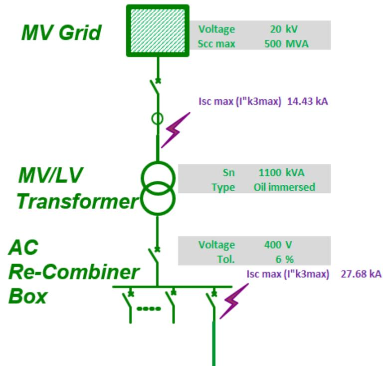
When we replace the 1100 kVA transformer with a 800 KVA transformer, the fault level decreases significantly on the AC re-combiner's bus bar and NSX400N type breakers become eligible to be used for inputs.
