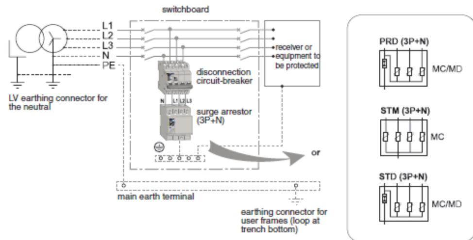
Figure 18 TN-C Earthing System, 3-Phase
