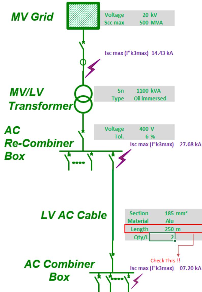
The example circuit in *Figure 10* has a 250 m length from the AC combiner to the AC re-combiner, and the fault current is reduced to 7.20 kA, allowing the selection of C120H MCB with 15 kA fault level.
