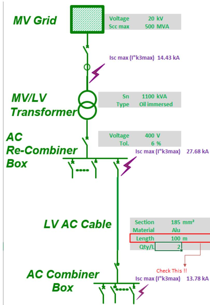
The example circuit in Figure 9 has 100 m length from the AC combiner to the AC re-combiner. The resulting fault level at the AC combiner bus bar is 13.78 kA and the choice of breaker is NG125N MCCB (25 kA).
