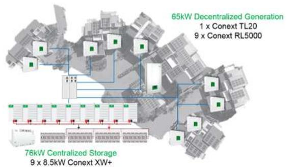
A bird's eye view showing the decentralized production with centralized storage architecture used on the One Everton Road project. The installation consists of a 76 kW battery based installation and 11 grid-tied inverters all connected to keep the development running off-grid
