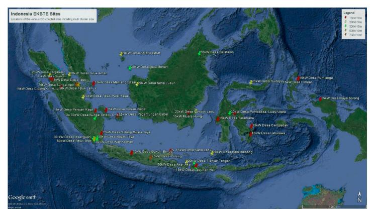
This image shows locations of the 60 systems that are being installed as part of the Indonesia EBTKE Rural Electrification Project. These systems range in size from 15kW to 75kW and are powered 100% from solar and battery storage.
