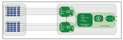
Figure 2-4 Standard block Option 4 for a 2MW system
