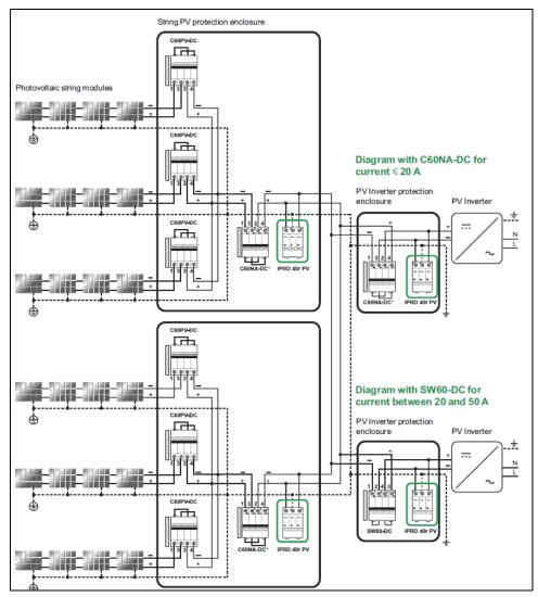
Figure 5-1 Installation of SPDs
