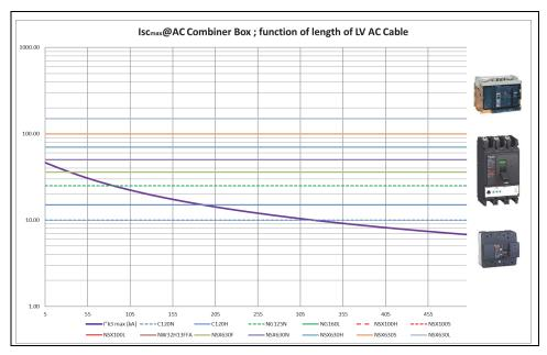
Figure 4-5 Isc<sub>max</sub> and length of the LV AC cable relationship
