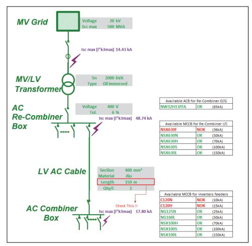
Figure 4-3 Example circuit with 150m cable
