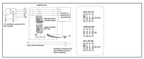
Figure 5-4 TN-S Earthing System, 3-Phase + Neutral
