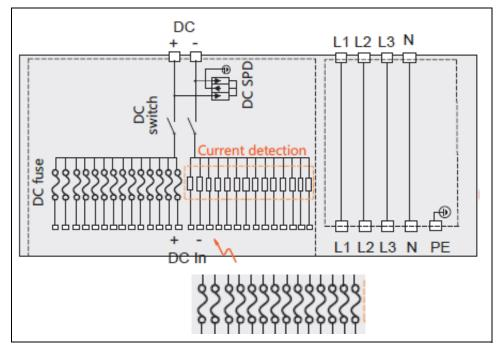
Figure 3-1 Wiring Box circuit diagram of the CL-60E inverter
