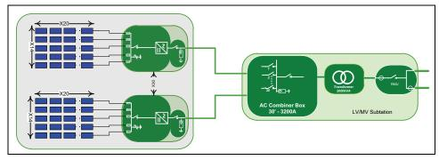
Figure 2-3 Standard block option 3 for a 2MW system
