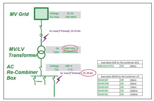
Figure 4-8 Breaker selection with 1000 kVA transformer
