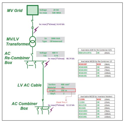
Figure 4-4 Example circuit with 250m cable
