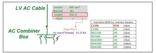
Figure 4-6 Choice of circuit breakers with calculated fault current
