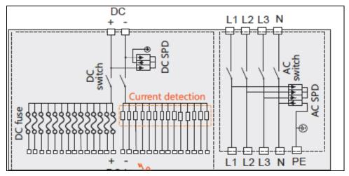
Figure 5-3 Circuit of Internal SPD Connections
