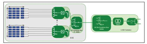
Figure 2-2 Standard block option 2 for a 2MW system
