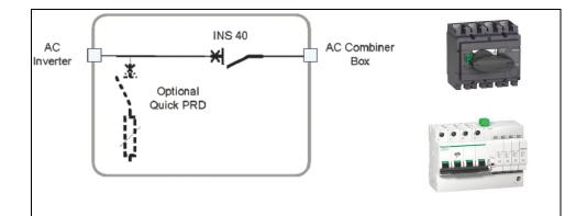
Figure 4-2 AC Switch Box Schematic Diagram
