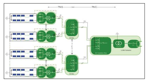
Figure 5-8 Grounding Circuit Connections
