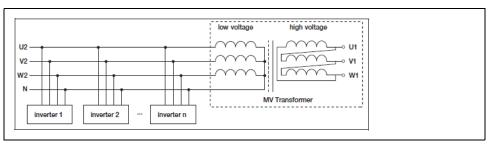
Figure 5-9 Parallel connection of multiple inverters to transformer winding
