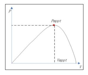
MPPT voltage range 570 ~ 950V Full MPPT voltage range :570 ~ 850V Maximum voltage 1000V; Starting voltage 620V
