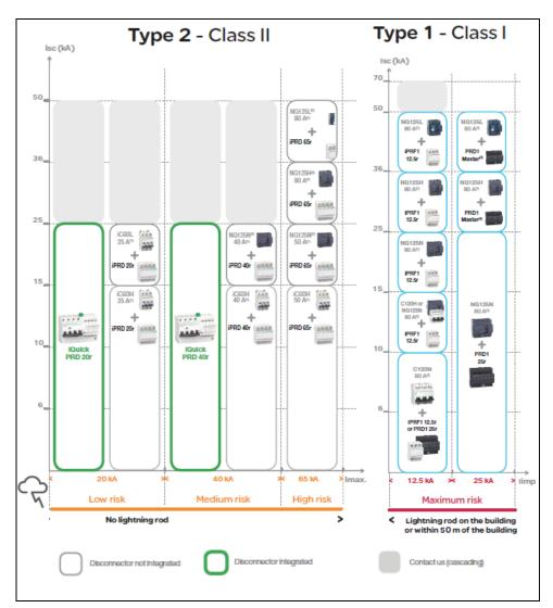
Figure 5-2 Coordination of SPDs with disconnection devices
