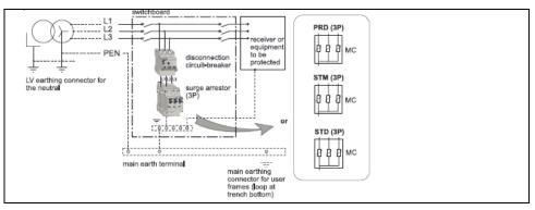
Figure 5-5 TN-C Earthing System, 3-Phase
