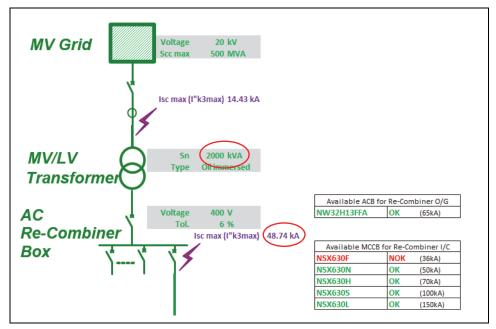
Figure 4-7 Breaker selection with 2000 kVA transformer
