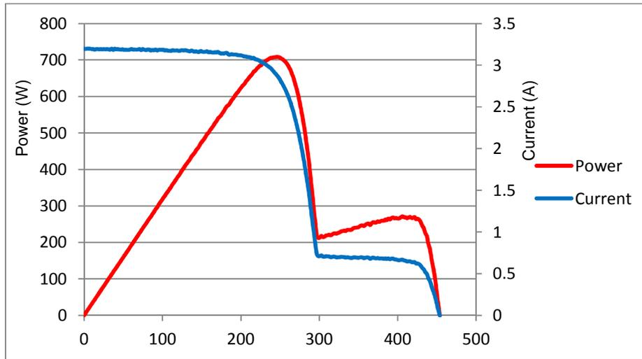
At the global maximum power point (MPP), the power harvested (P1) is 705W at voltage of 245V.
