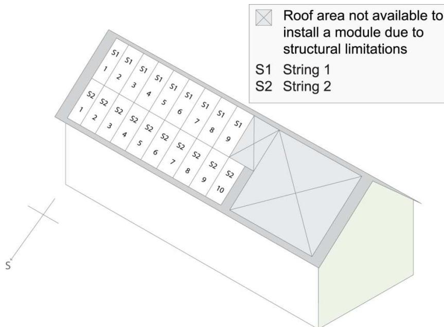
As represented above, the entire roof area is not available for the solar PV installation due to structural limitations. Assuming the plant owner is willing to install a typical 220 W polycrystalline module, the DC power rating of the first string (S1) with 9 modules becomes 1980W and that of the second string (S2) with 10 modules becomes 2200W.
