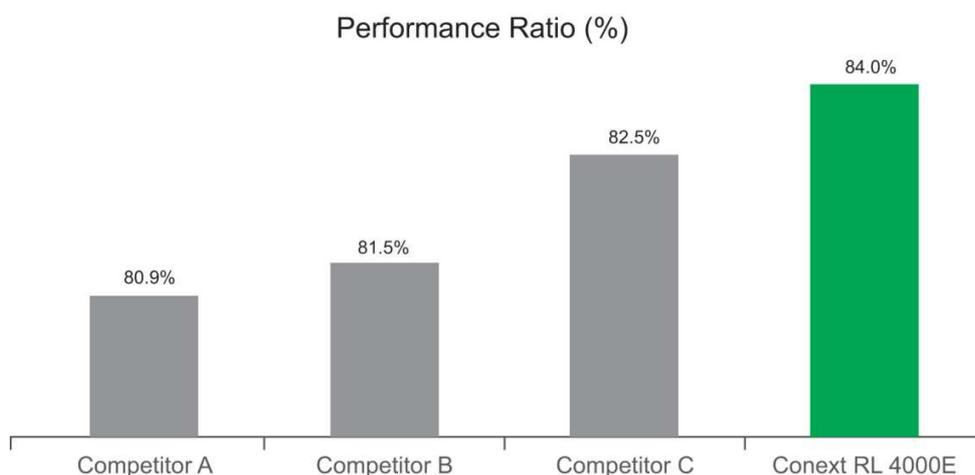
Performance ratio (PR) represents the ratio of the effectively produced energy and the energy which would be produced by a "perfect" system continuously operating at STC under same irradiance. The PR calculation includes the array losses (shadings, module quality, mismatch, wiring, etc.) and the system losses (e.g., inverter efficiency).
