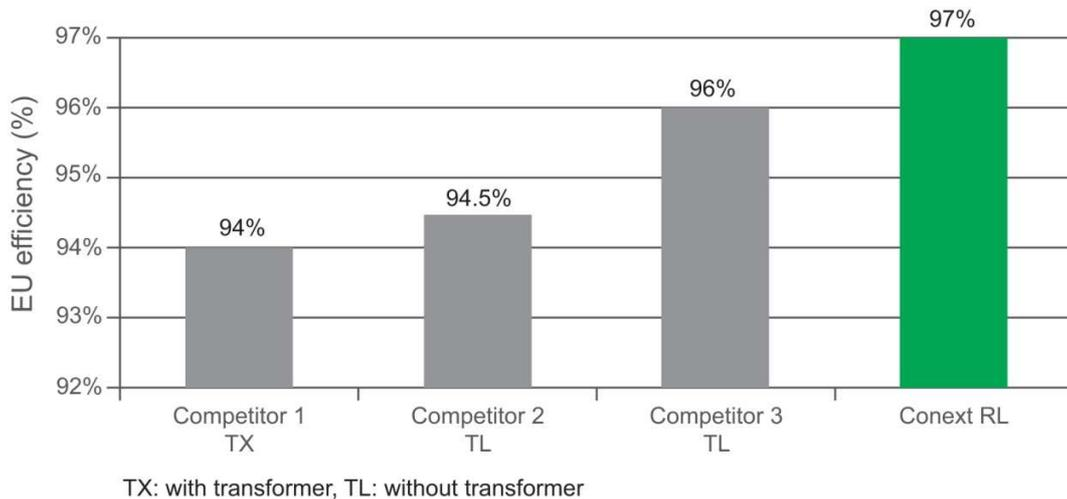
As represented in Figure 2 above, higher efficiency of Conext RL facilitates the harvest of 1-3% additional energy than a representative competitor inverter.
