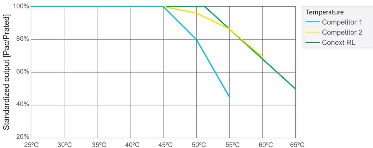
At ambient temperature of 50°C Conext RL harvests 100% of the rated output power. Competitor 1 unit harvests 80% of the rated output power while Competitor 2 unit harvests 95% of the rated power.
