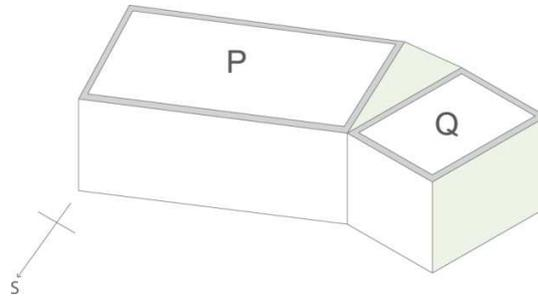
A typical single MPPT inverter does not have an ability to handle unbalanced array I/Ps and hence it cannot be used to accept both strings from roof areas 'P' and 'Q' as the inputs. With such an inverter you have two options:
