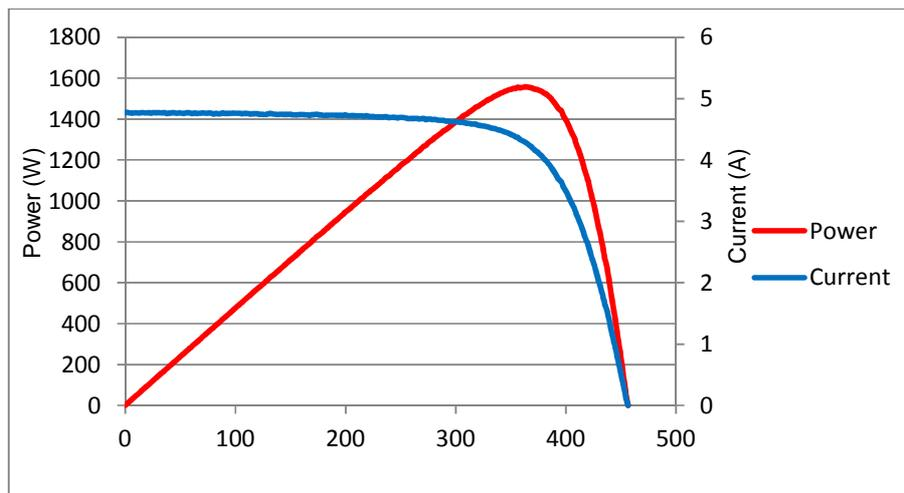
At the maximum power point (MPP), the power harvested (P2) is 1550W at voltage of 335V.
