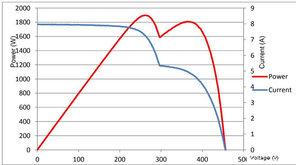
Depending on the effectiveness of the shade tolerant algorithm, the power corresponding to either the local or the global maxima will be harvested. The best case power harvested in the installation 1 is 1900W at 263V. If the MPPT algorithm of the inverter is not effective, the power harvested can be even lower, i.e., 1810W at 365V.
