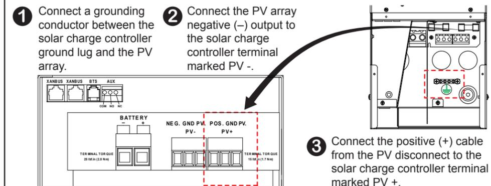
For details, see the *Conext MPPT 80 600 Solar Charge Controller Installation Guide (975-0540-01-01)*.
