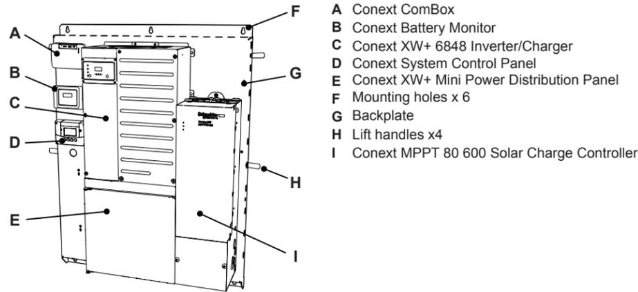
NOTE: All components except the lift handles are supplied pre-assembled.
