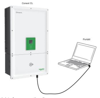
Figura 2-55 Web interface connection diagram
