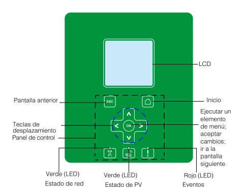
Figura 3-1 Panel de control LCD
