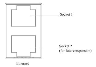
Figure 2-46 Ethernet Connection
