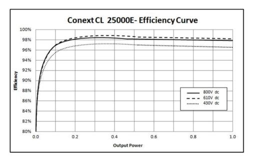
Figure A-2 Efficiency curve- 25kW
