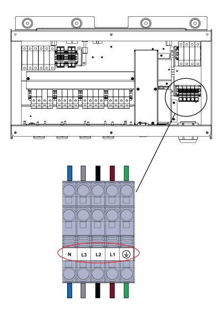
Figure 2-36 Wire installation
