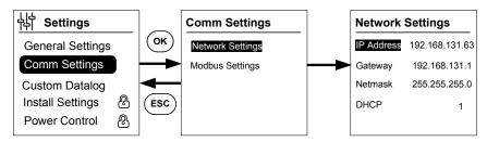
Figure 2-45 Checking the IP address
