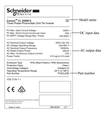
Figure 2-5 Inverter nameplate label
