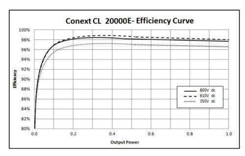
Figure A-1 Efficiency curve - 20kW
