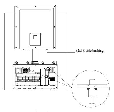
Figure 2-29 Inverter assembly- front view
