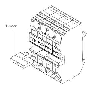
Figure 2-34 MPPT Shorting Connector and Jumper arrangement
