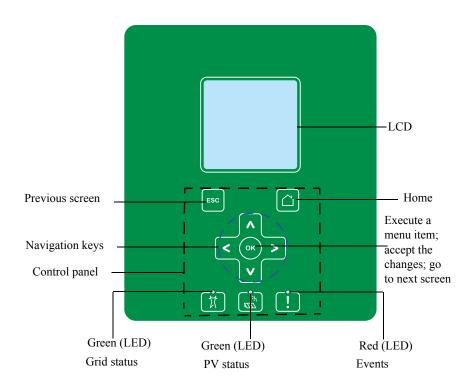
Figure 3-1 LCD Control Panel
