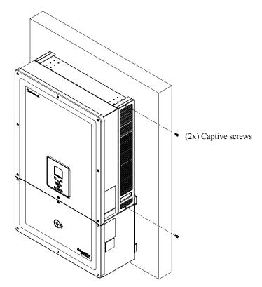
Figure 5-1 Loosening the louver cover- right side
