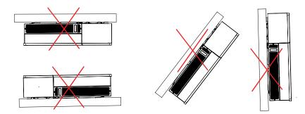
Figure 2-7 **Incorrect mounting positions**
