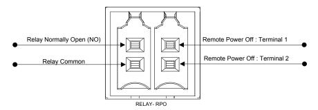
Figure 2-50 RPO and Relay Contact terminal details
