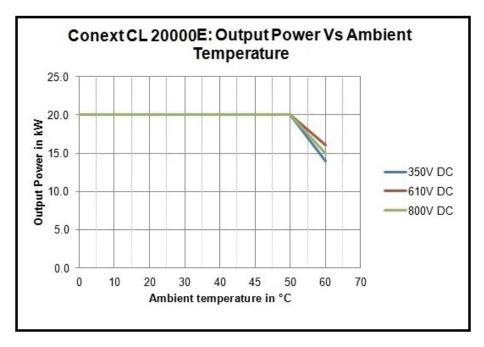
Figure A-3 Derating curve- 20kW
