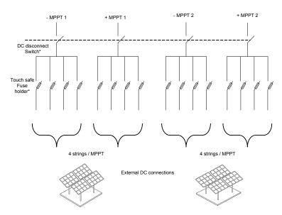
Figure 2-33 PV Wiring diagram of Conext™ CL 20000E and 25000E models
