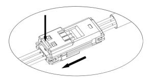
Figure 5-8 Unlocking the fan connector tabs
