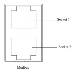
Figure 2-44 Modbus (RS485) connectors
