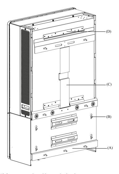
Figure 2-18 Inverter rear view with mounting bracket
