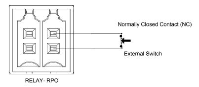
Figure 2-53 **RPO connection for single inverter**
