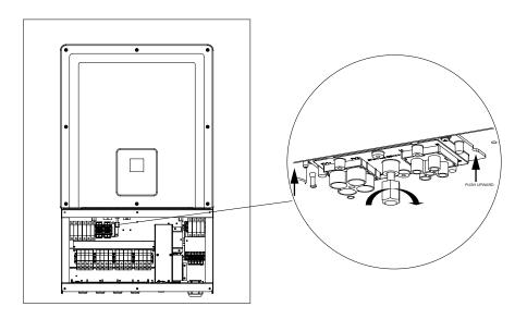
Figure 2-31 Locking Inverter and Wiring box power connector
