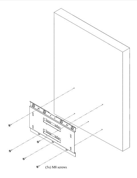
Figure 2-16 Fastening the wiring box mounting plate to the wall
