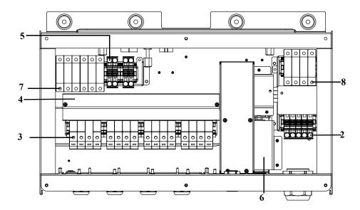
Figure 2-13 Wiring box- Optimum (PVSCL2025E300)
