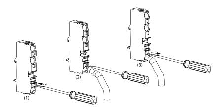
Figure 2-37 Wire installation
