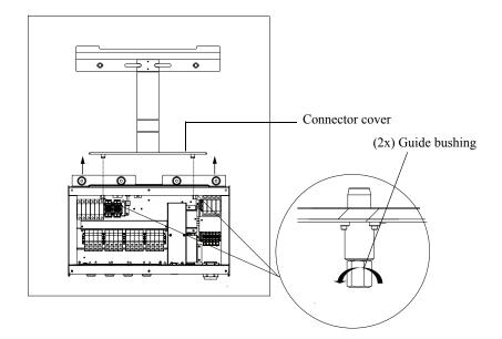
Figure 2-26 Removing the connector cover
