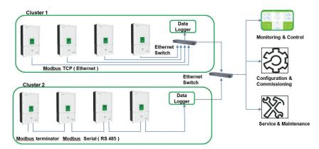
Figure 2-49 Cluster 1: Modbus TCP and Cluster 2: Modbus RS485 connections
