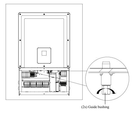
Figure 2-30 Locking the inverter to the wiring box
