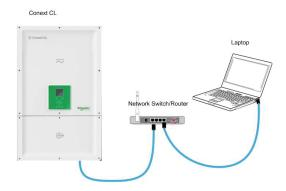
Figure 2-58 Web Interface connection via router diagram
