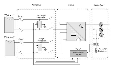
Figure 2-55 Surge Protection device wiring
