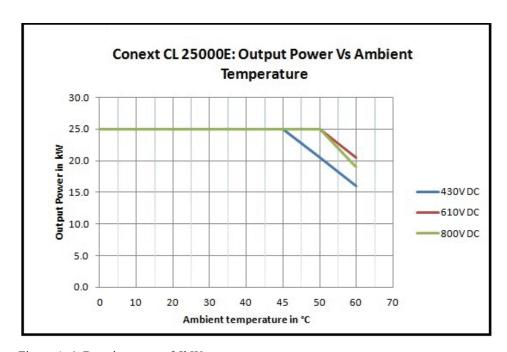
Figure A-4 Derating curve- 25kW
