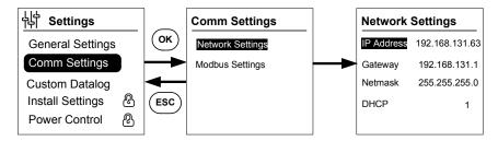
Figure 2-56 Checking the IP address
