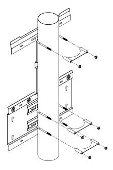
Figure 2-20 Rear view of the pole mounting installation
