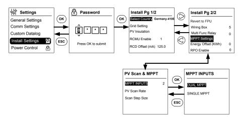
Figure 2-35 MPPT settings through Install settings menu
