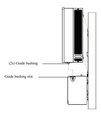
Figure 2-28 Inverter assembly- side view
