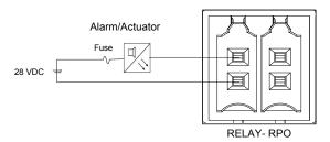
Figure 2-51 Dry Contact Relay connection
