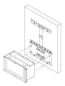
Figure 2-23 Mounting the wiring box on the bracket
