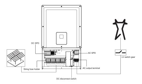
Figure 1-1 Typical Installation (Optimum plus Configuration)
