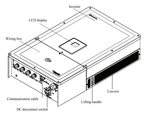
$\label{eq:Figure 1-3} \textbf{Location of physical features of the inverter and the wiring box-right side } \\ \textbf{view}$
