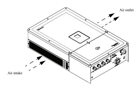
Figure 1-5 Cooling arrangement of the inverter
