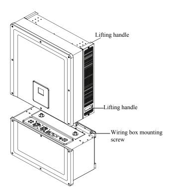
Figure 2-22 Inverter and Wiring box- Exploded view
