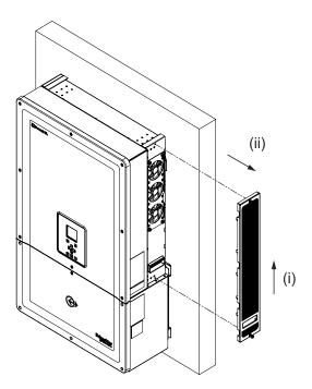
Figure 5-3 Removing the louver cover- right side
