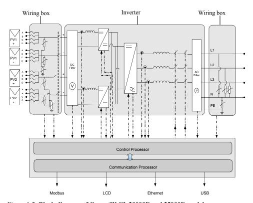
Figure 1-2 Block diagram of Conext™ CL 20000E and 25000E models
