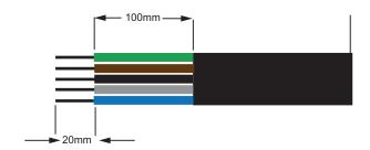
Figure 2-39 AC wiring
