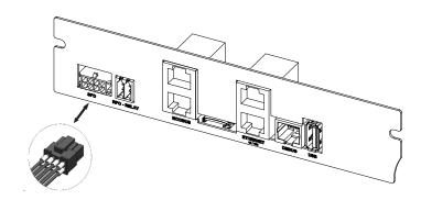
Figure 2-43 SPD monitoring cable connection
