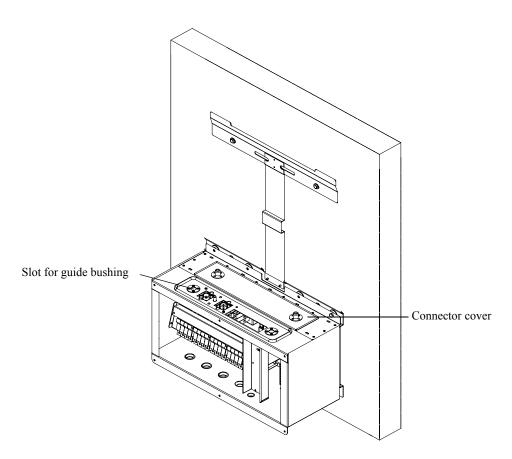
Figure 2-27 **Anchoring the connector cover**
