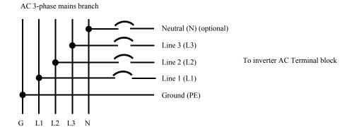
Figure 2-38 AC connection details
