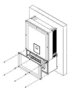
Figure 2-32 Closing the wiring box
