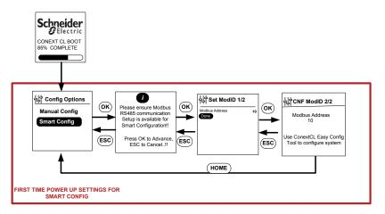
Figure 3-4 First Time Power Up: Smart Config screen
