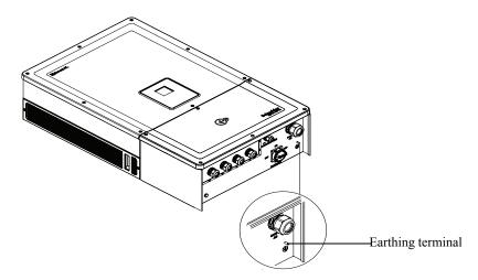
Figure 2-40 Connecting the earthing conductor
