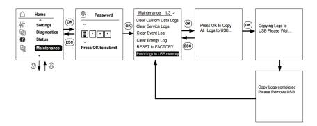
Figure 4-1 Pushing Logs to USB flash Device
