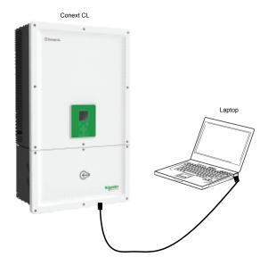
Figure 2-57 Web Interface connection diagram
