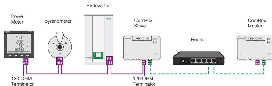
**Figure 1** Daisy-Chain RS-485 Network Illustration
