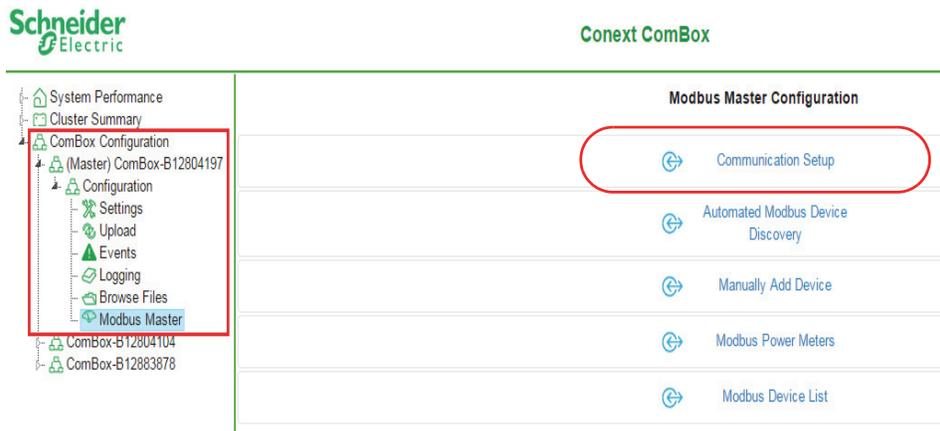
**Figure 14** Modbus Master Configuration Page
