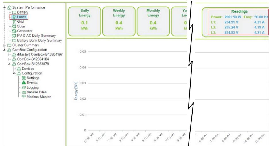
Figure 19 Loads page displaying Power Meter readings
