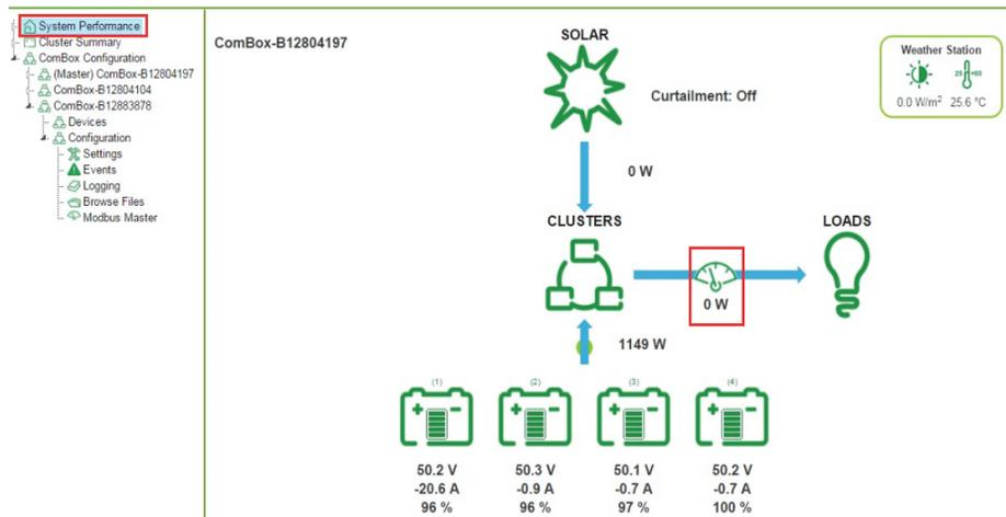
**Figure 18** System Performance page displaying Power Meter
