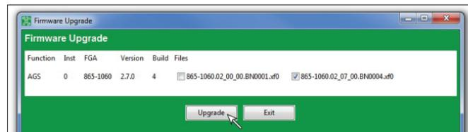
**NOTE:** Progress bars for each device will be displayed below the panel, as well as an overall progress bar. Firmware is upgraded on one device at a time. No firmware changes are made to a device until the previous device is fully upgraded.
