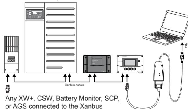
**NOTE:** Any XW+, CSW, Battery Monitor, SCP, or AGS connected to the Xanbus network may be updated.
