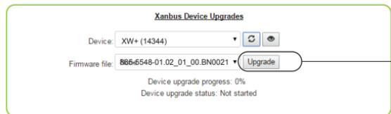
Click to confirm you have selected the device you want. Click to activate a visual (such as a flashing LED) and/or audio (such as in AGS) indicator on the selected device.
