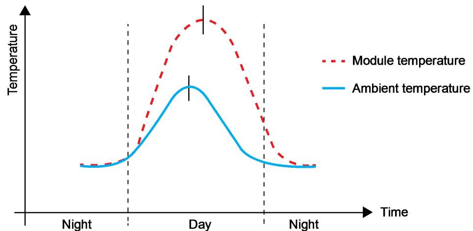
The temperature difference between the ambient air and the modules depends on the solar irradiance and other climatic factors like wind.
