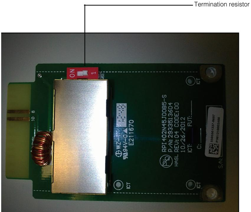
Figure 2-39 Termination resistor—switch numbering
