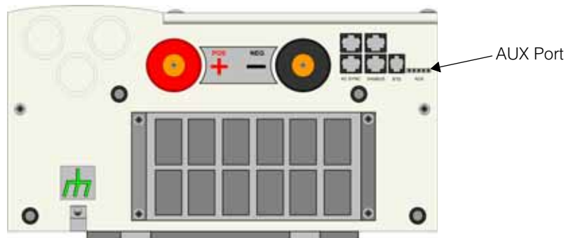
Figure 2-16 AUX Port Location
