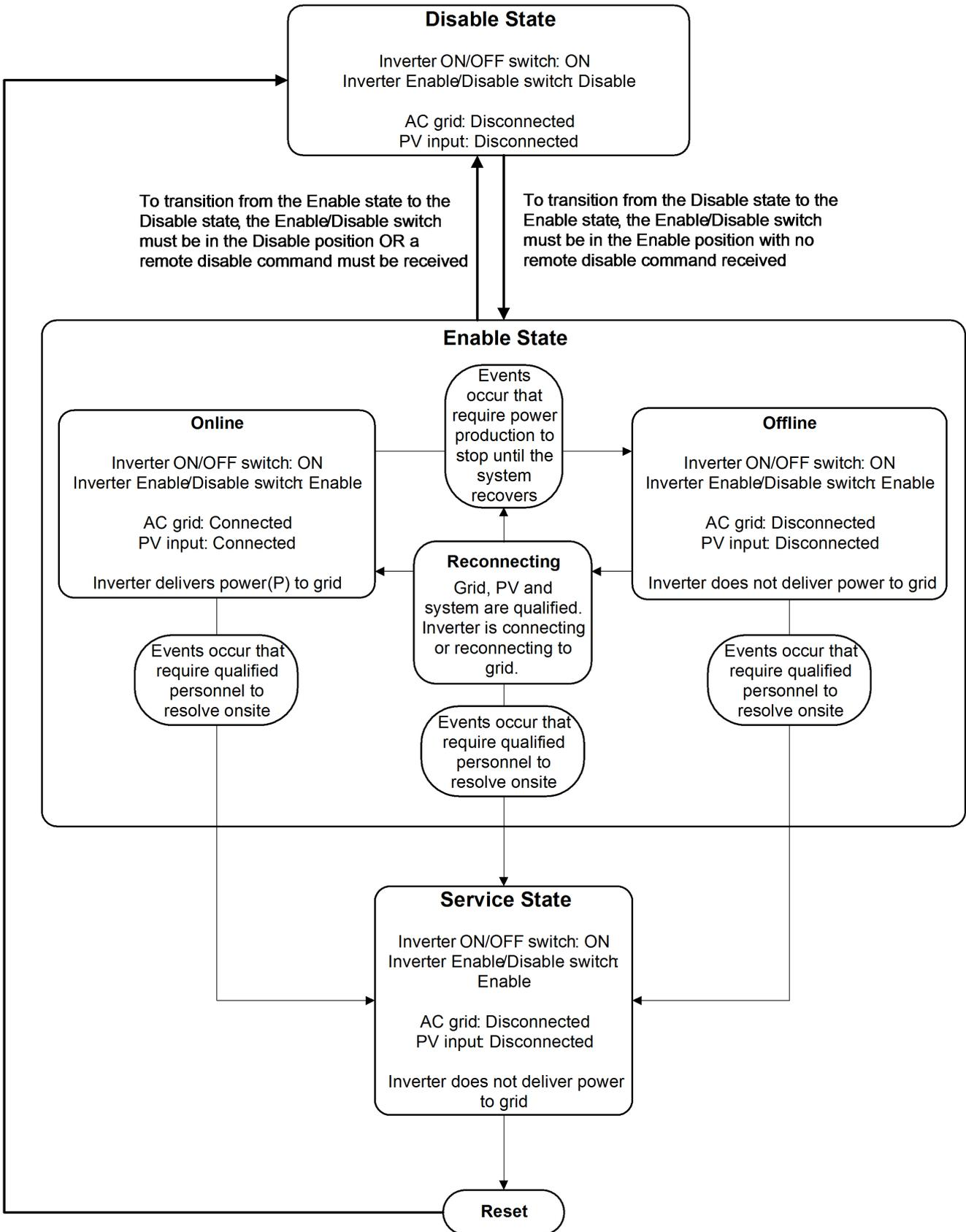
Figure 7 Conext Core XC Series operational states in PVCQ mode
