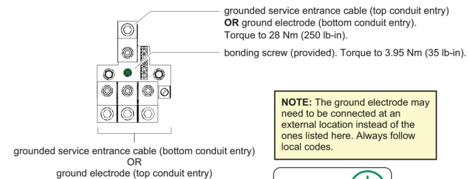
**NOTE:** The ground electrode may need to be connected at an external location instead of the ones listed here. Always follow local codes.
