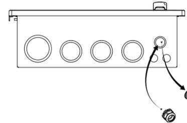
5 Starting with the far right conduit hole, install conduit fittings (suitable for desired ingress rating).
